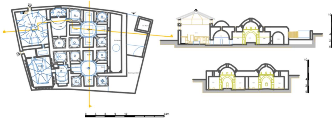
Figure 2. The architectural survey (measured drawing) of Mustafa Aga bath 'hamam'.
