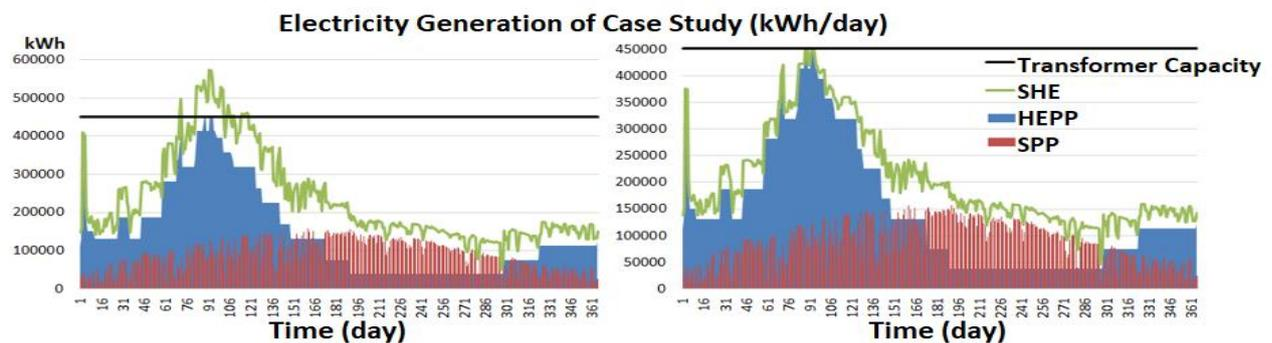
Fig. 11. The electricity generation of the regular flow based SHE system (2nd scenario)
