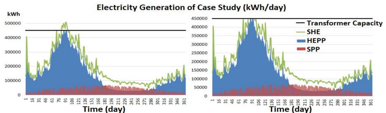
Fig. 9. The electricity generation of the irregular flow based SHE system (1st scenario)
