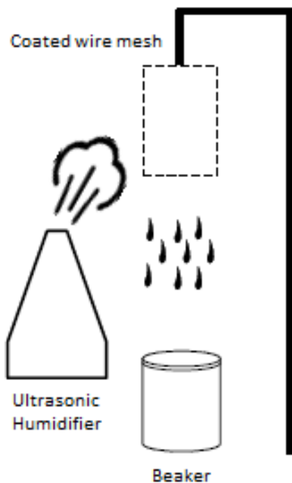
Figure 2. Experimental setup for water harvesting capacity test
