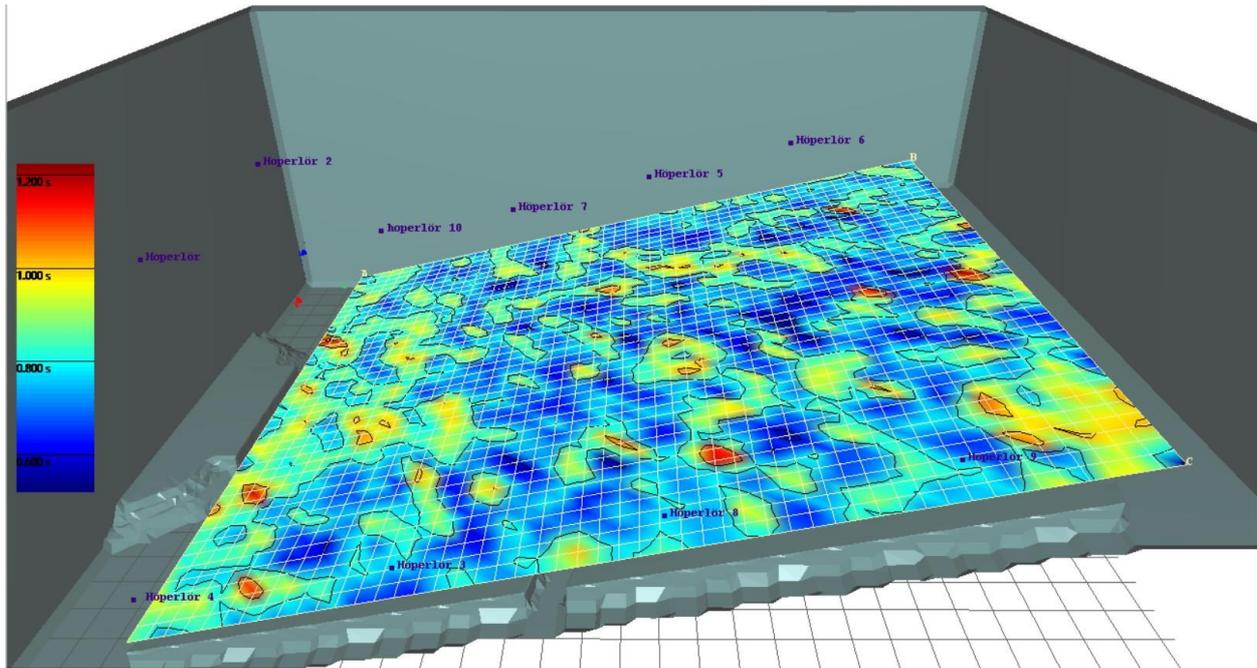
**Figure 14.** In the I-SIMPA software, the main lecture hall reverberation time results ( $T_{15}$ ) at 500 Hz
