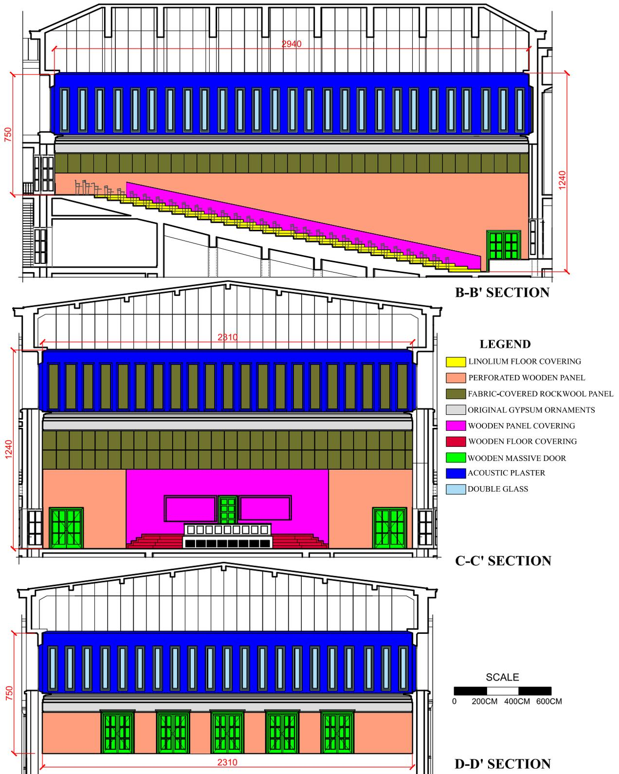
*Figure 11. Acoustic coating project of the main lecture hall, B-B', C-C' and D-D' sections*
