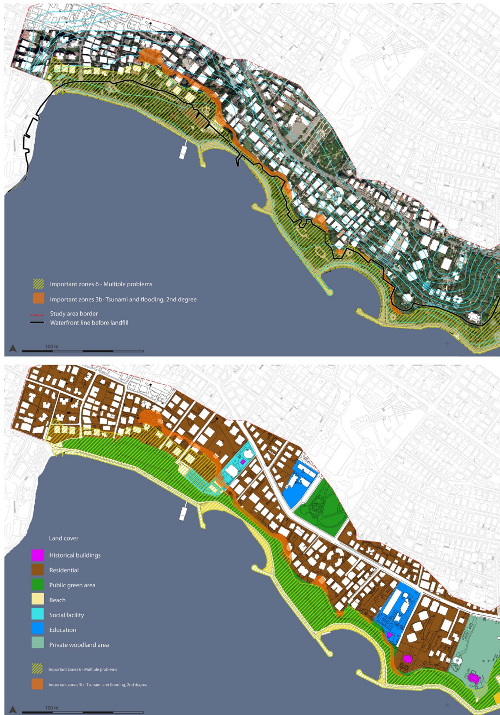
Figure 3: Overlay maps showing risk areas, topography with contours every 1m (top), and land cover (bottom) in Zone 1
