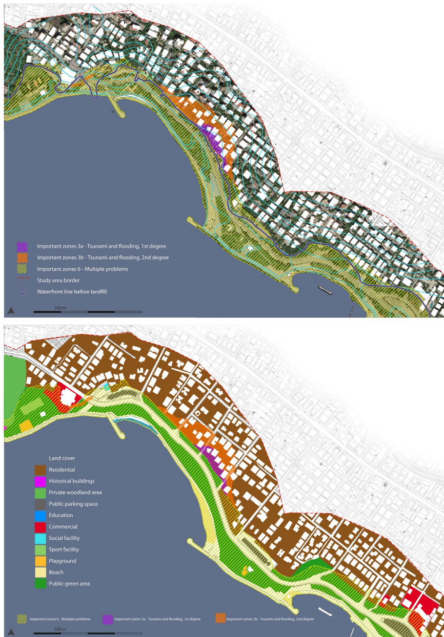
Figure 4: Overlay maps showing risk areas, topography with contours every 1m (top), and land cover (bottom) in Zone 2
