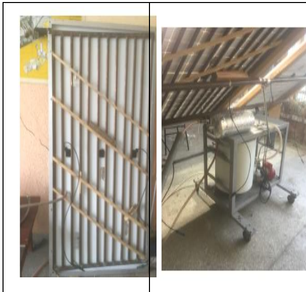
Figure 2. The cooling circuit
