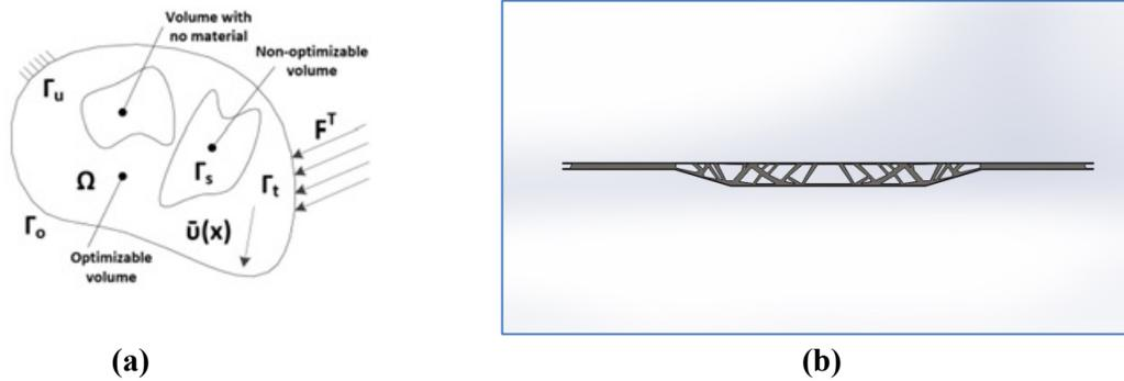
**Figure 4.** (a) Generalized shape design problem of finding the optimal material distribution in the 3D domain, and (b) Topology optimization part
