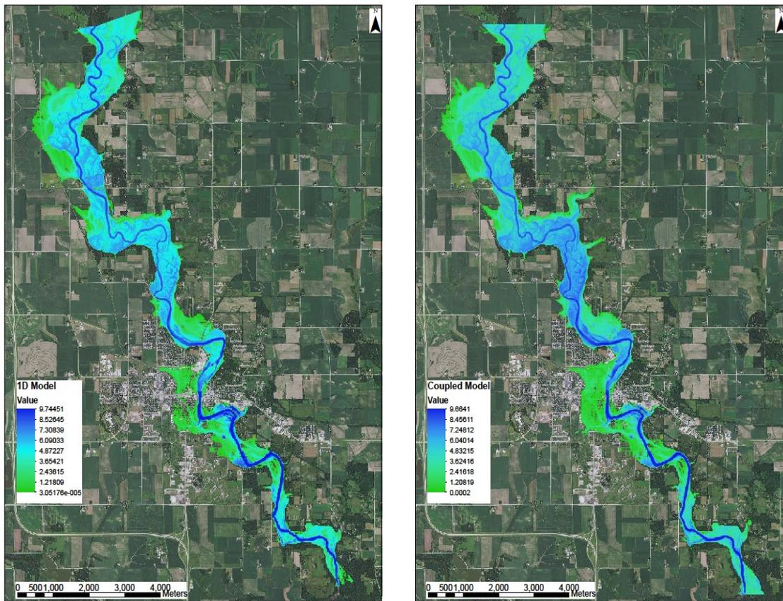
Figure 7. 2008 flood inundation maps using Calibrate 1D and Coupled Model
