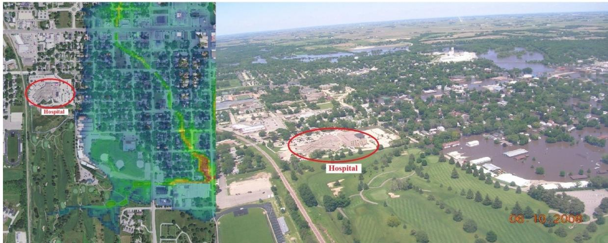
Figure 9. Comparison of 2008 flood inundation between airphoto and coupled model result-2
