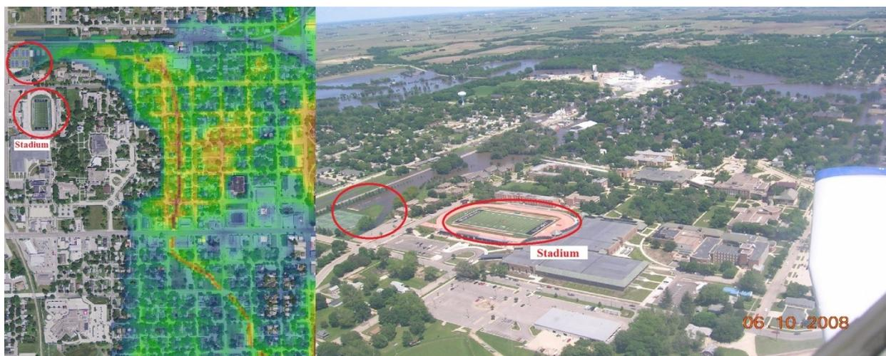
Figure 8. Comparison of 2008 flood inundation between airphoto and coupled model result-1
