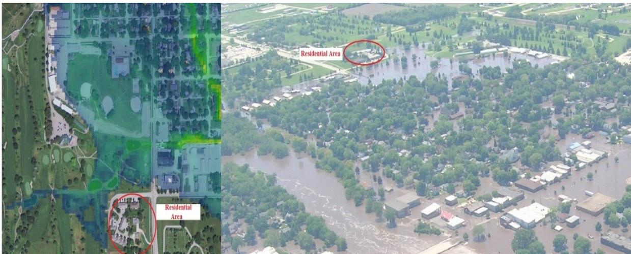
Figure 10. Comparison of 2008 flood inundation between airphoto and coupled model result-3
