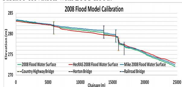
Figure 6. 1D and Coupled model calibration using highwater levels on river bed
