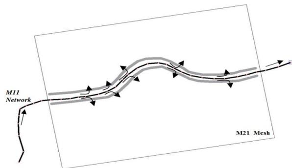
Figure 1. Lateral link structure between one-dimensional MIKE 11 and two-dimensional MIKE 21 [17]
