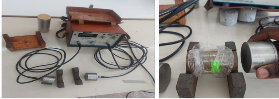
**Figure 5.** The appearance of the specimen during the UPV test.
