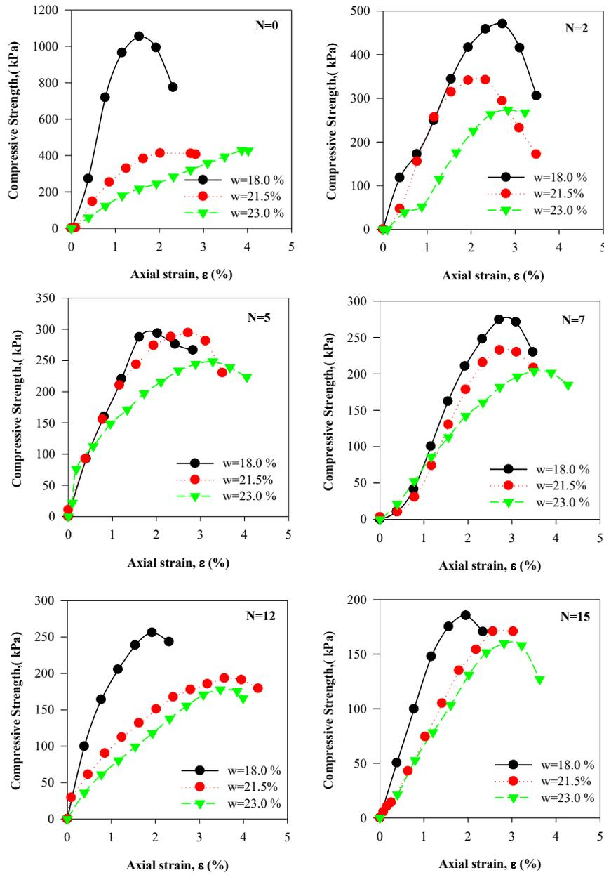
Figure 6. The UCS versus axial strain of the specimens for different  $w$  and  $N$ .
