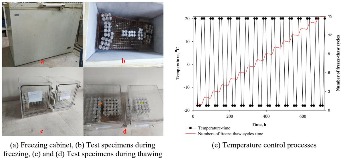
Figure 3. Freeze-thaw tests.
