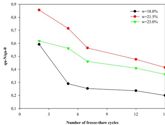
**Figure 8.** Variation of  $q_u-N/q_{u-0}$  ratio with freezing-thawing cycles for different  $w$ .
