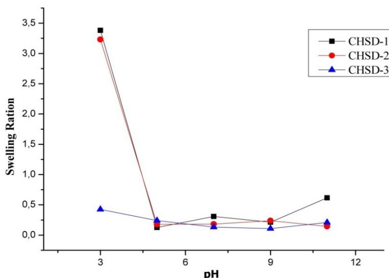
**Figure 6:** Effect of pH on the degree of swelling of the CHSDs.
