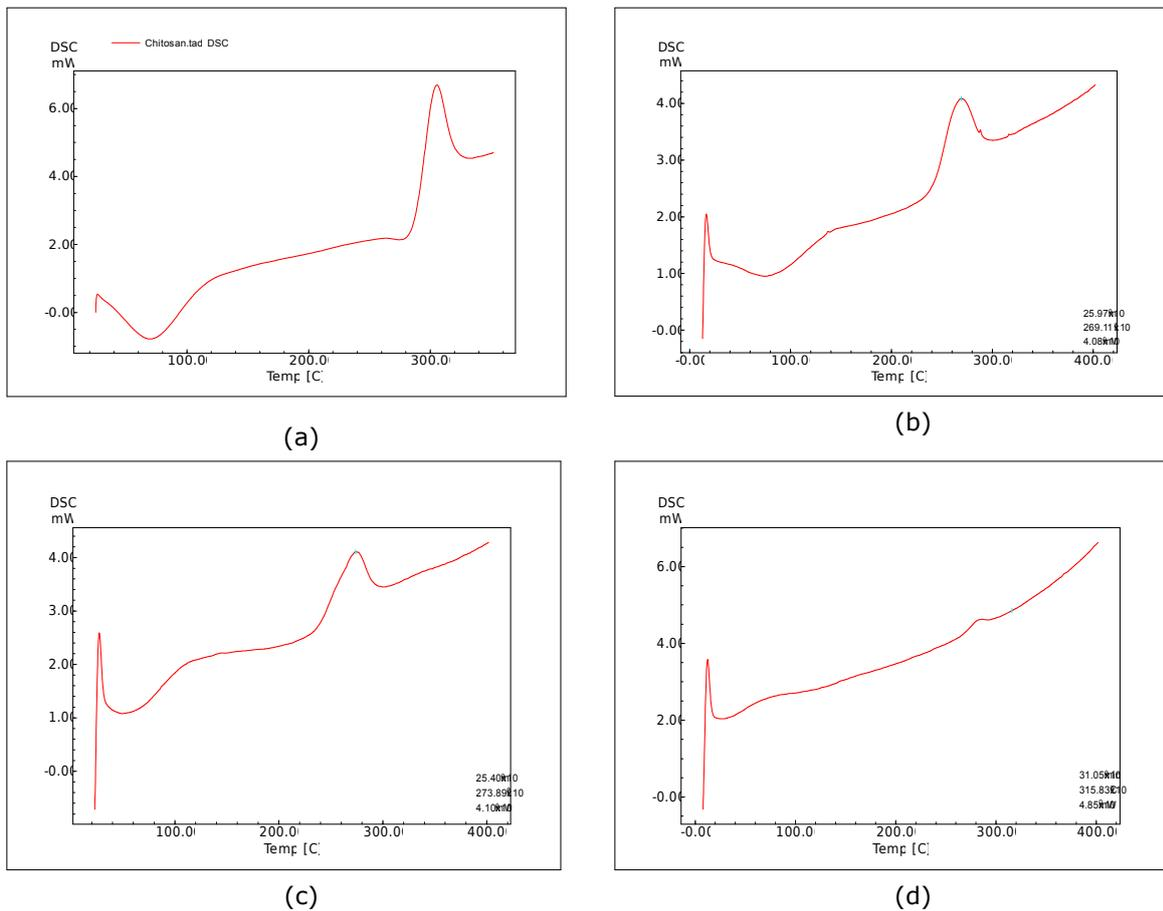
Figure 4: DSC thermogram of CHSDs (a:CH, b:CHSD1, c:CHSD2, d:CHSD3).
