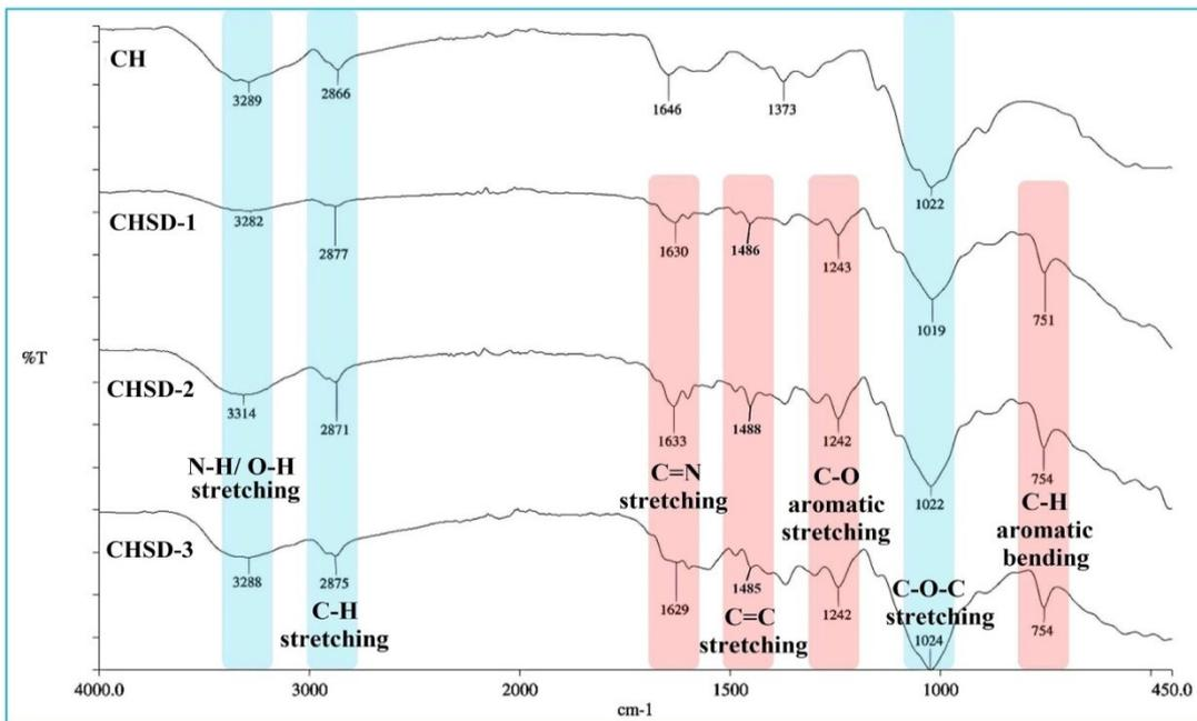
**Figure 2:** IR spectra of CH and CHSD1-3.
