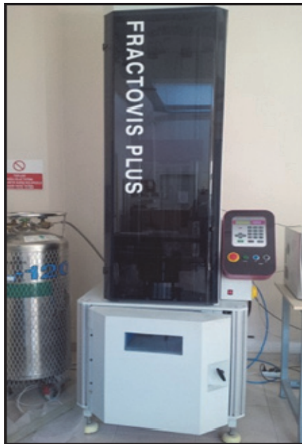
Figure 3. Experimental setup of the low velocity impact test
