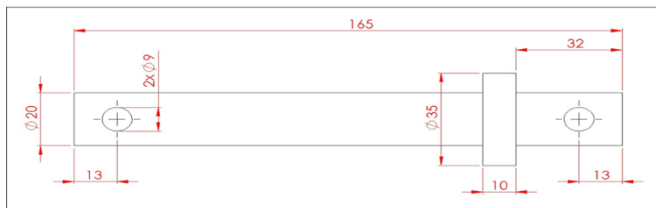
Figure 1. Technical drawing of safety pin
