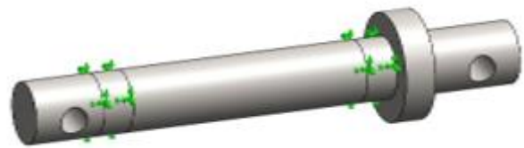
Figure 3. Surfaces fixed in bending analyzes
