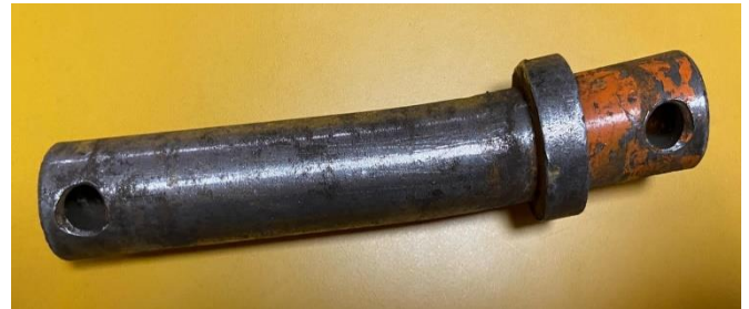
Figure 2. Bending condition of the safety pin after use
