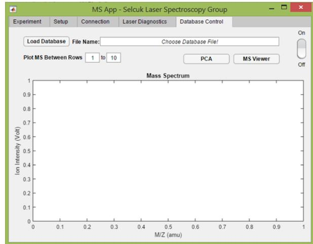
**Figure 3.** Database control section consists MS viewer button and a statistical analysis button to perform PCA.
