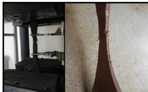
Figure 12. Tensile test image of the unspliced belt
