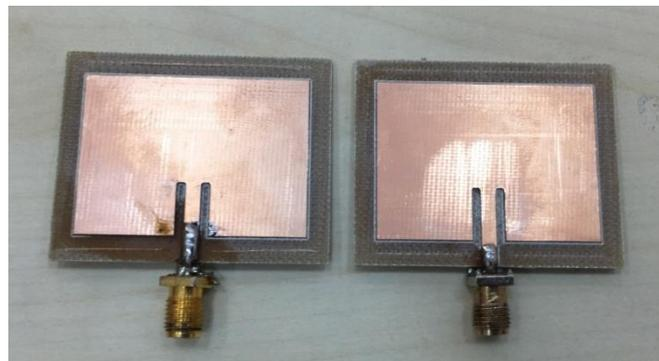
**Figure 3.** Fabricated antennas
