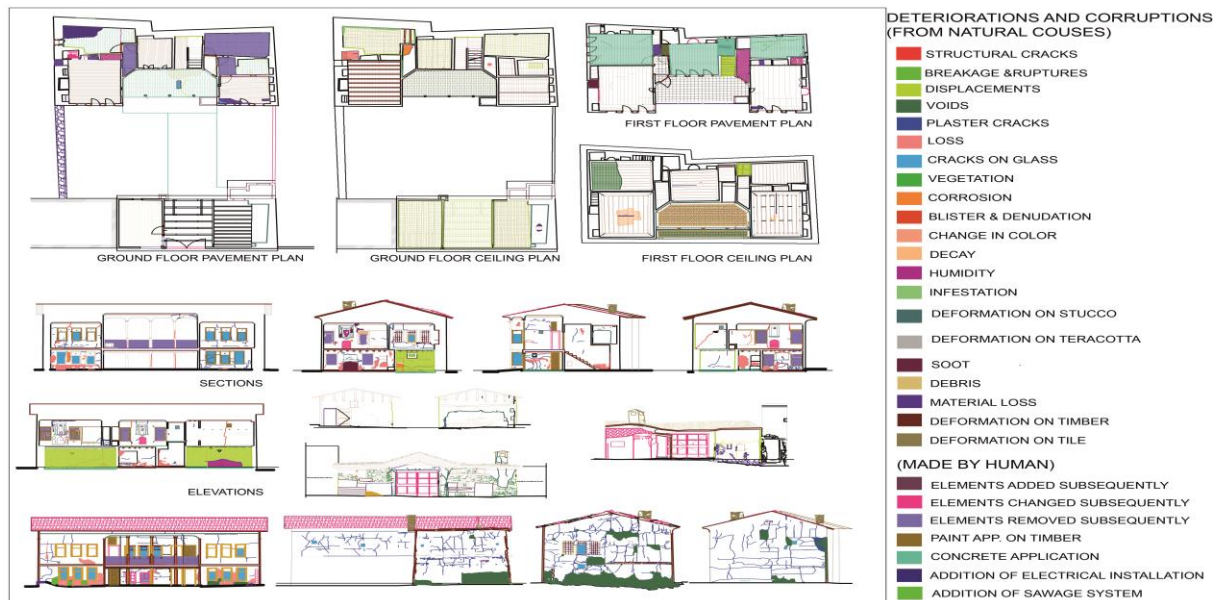
Figure 5. Deteriorations and corruptions determined in Satıcı dwelling
