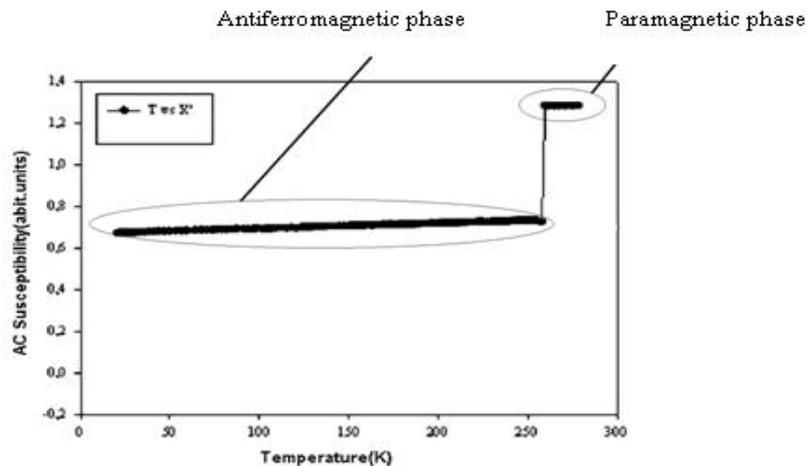
Figure 3. Magnetic susceptibility against temperature curves of Fe-13.2%Mn-5.3%Co alloy.
