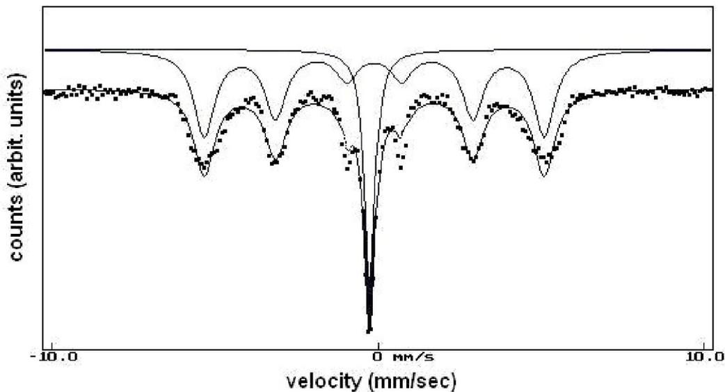
Figure 2. Room temperature Mössbauer spectra for quenched Fe-13.2%Mn-5.3%Co alloy. (Single pick: Austenite phase, Six pick: Martensite phase).
