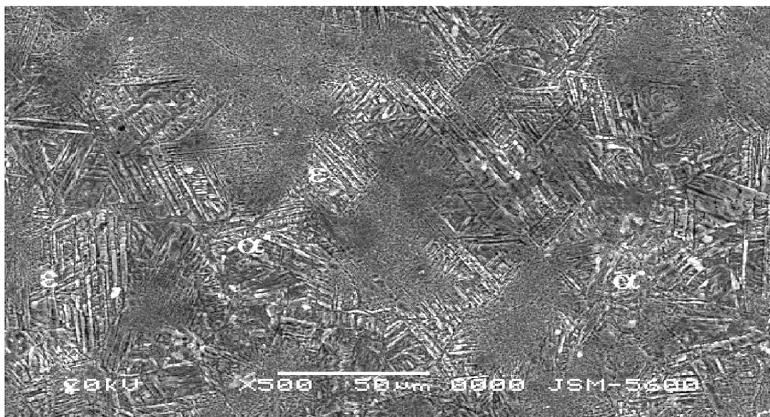
Figure 1. SEM micrographs showing the microstructure of quenched Fe-Mn-Co alloy.
