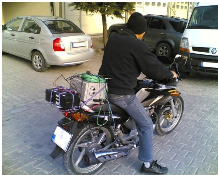
Figure 14. Data collection from the axle.
