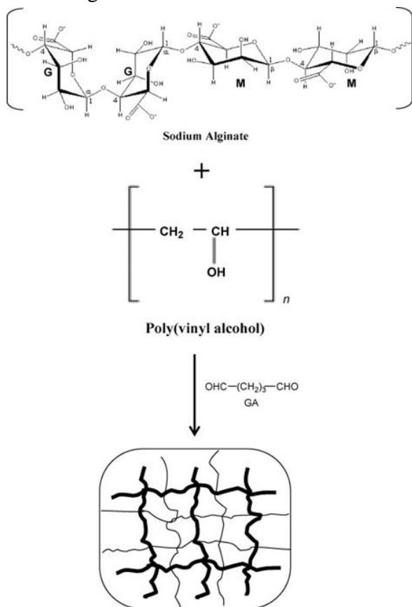
Figure 2 Schematic representation of the prepared crosslinked PVA/NaAlg [25]
