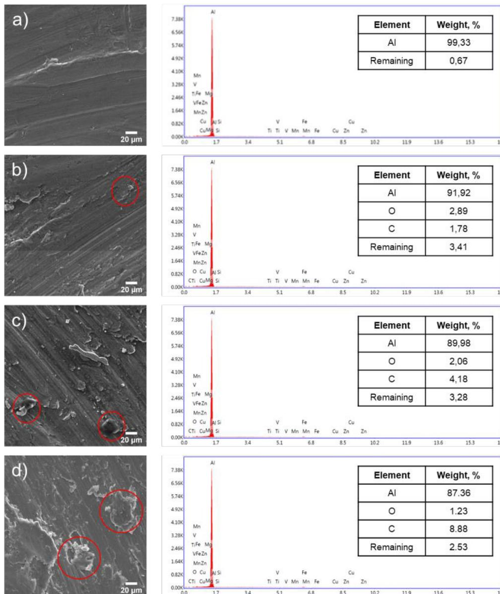
Figure 5. SEM and EDS analysis of pure and rGO added AA1070 samples
