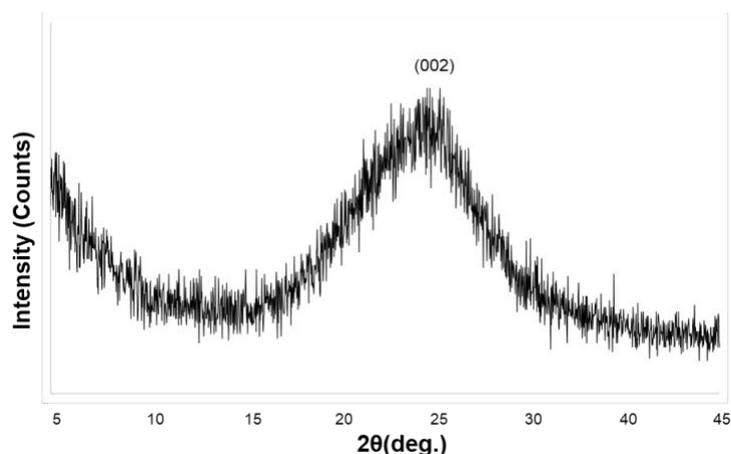
Figure 1. XRD analysis of synthesized rGO powder
