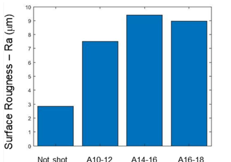
Figure 3. Average surface roughness of selected 0.25%wt. of rGO added AA1070 samples under different Almen intensity
