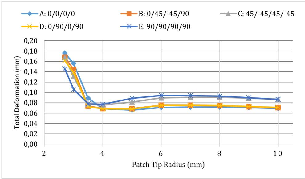
**Figure 12.** The total deformations calculated for varied composite patch tip radiuses and patch fiber orientations
