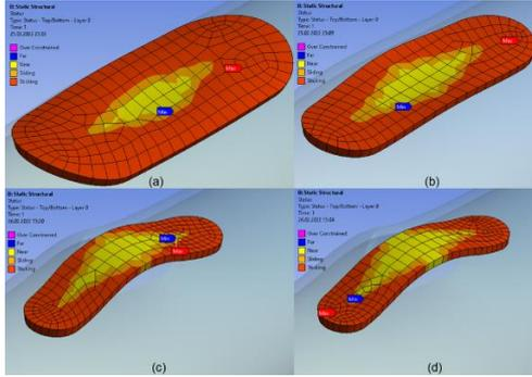
**Figure 9.** Bonded contact status between repairing patch and slotted specimen after applied pressure: Patch Code: a) C6, b) C4, c) C2, d) C1
