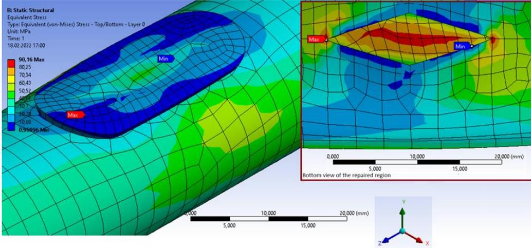
**Figure 7.** Equivalent stress distribution on patched up region of composite tube under internal pressure: Patch Code: C6
