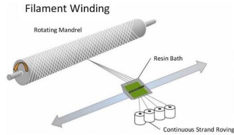
**Figure 1.** Schematic illustration of filament winding process [14]
