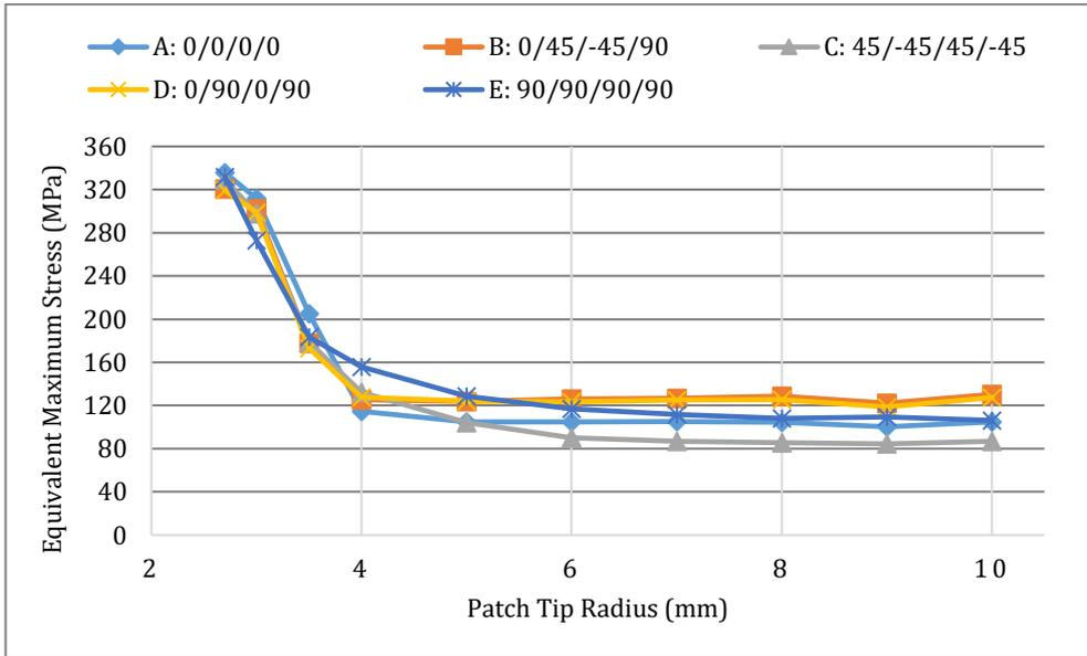
**Figure 11.** The equivalent maximum stresses calculated for varied composite patch tip radiuses and patch fiber orientations
