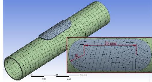
**Figure 3.** The dimensions of round tipped composite patch adhesively bonded on the specimen
