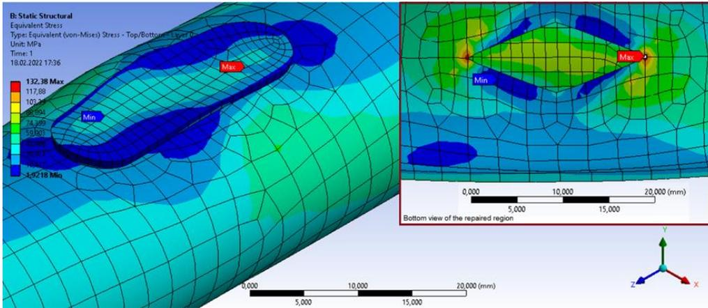
**Figure 8.** Equivalent stress distribution on patched up region of composite tube under internal pressure: Patch Code: C4
