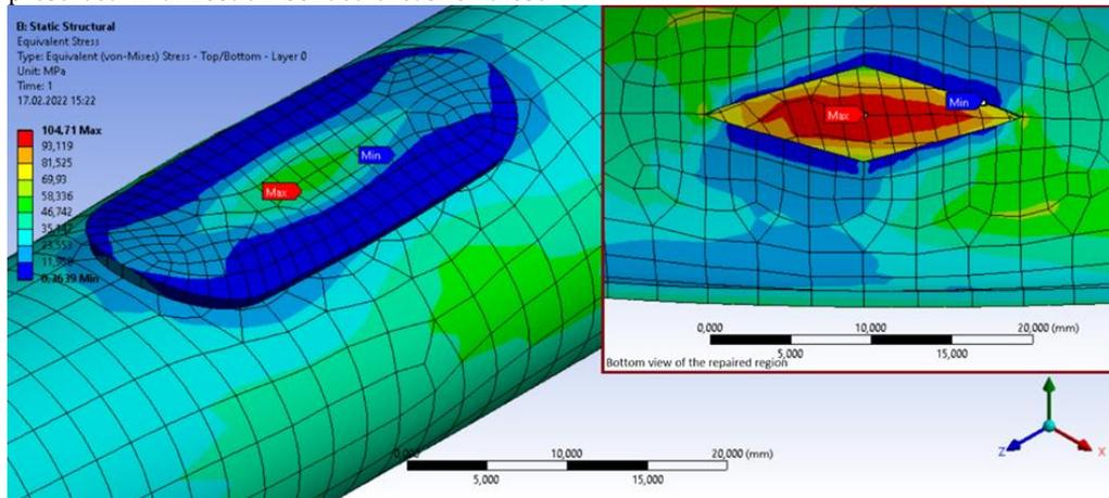
**Figure 4.** Equivalent stress distribution on patched up region of composite tube under internal pressure: Patch Code: A6
