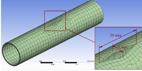
**Figure 2.** The dimensions of quadrilateral shaped slot on the specimen
