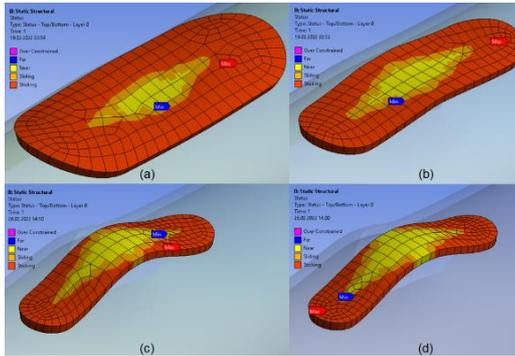
**Figure 6.** Bonded contact status between repairing patch and slotted specimen after applied pressure: Patch Code: a) A6, b) A4, c) A2, d) A1
