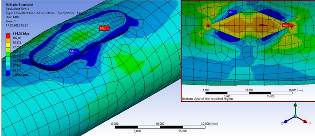
**Figure 5.** Equivalent stress distribution on patched up region of composite tube under internal pressure: Patch Code: A4
