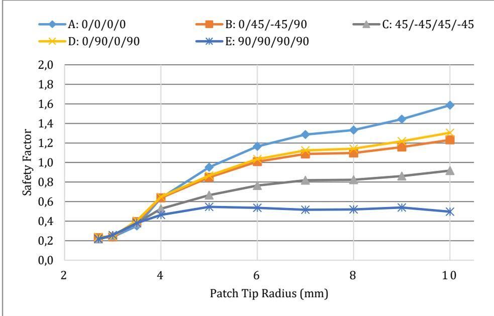
**Figure 10.** The factors of safety calculated for varied composite patch tip radiuses and patch fiber orientations
