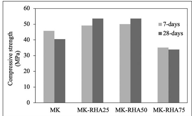
Figure 7. Compressive strength of geopolymer mortars at 7 and 28 days of ageing.
