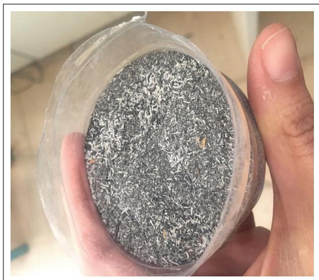
Figure 1. Burned rice husk ( $\geq 63 \mu\text{m}$ ).
