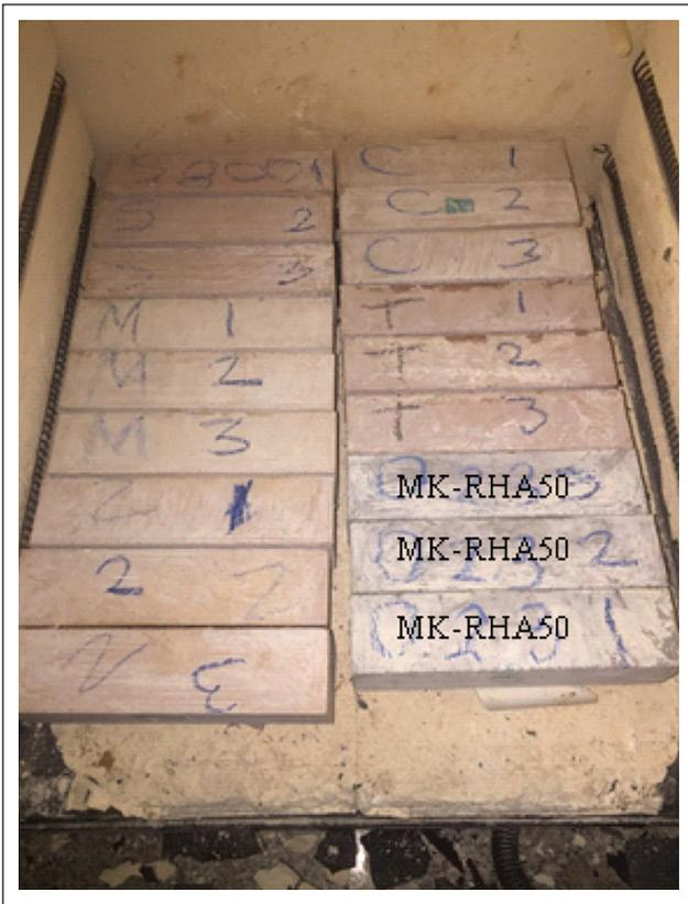
Figure 6. The prism specimens placed in the furnace.
