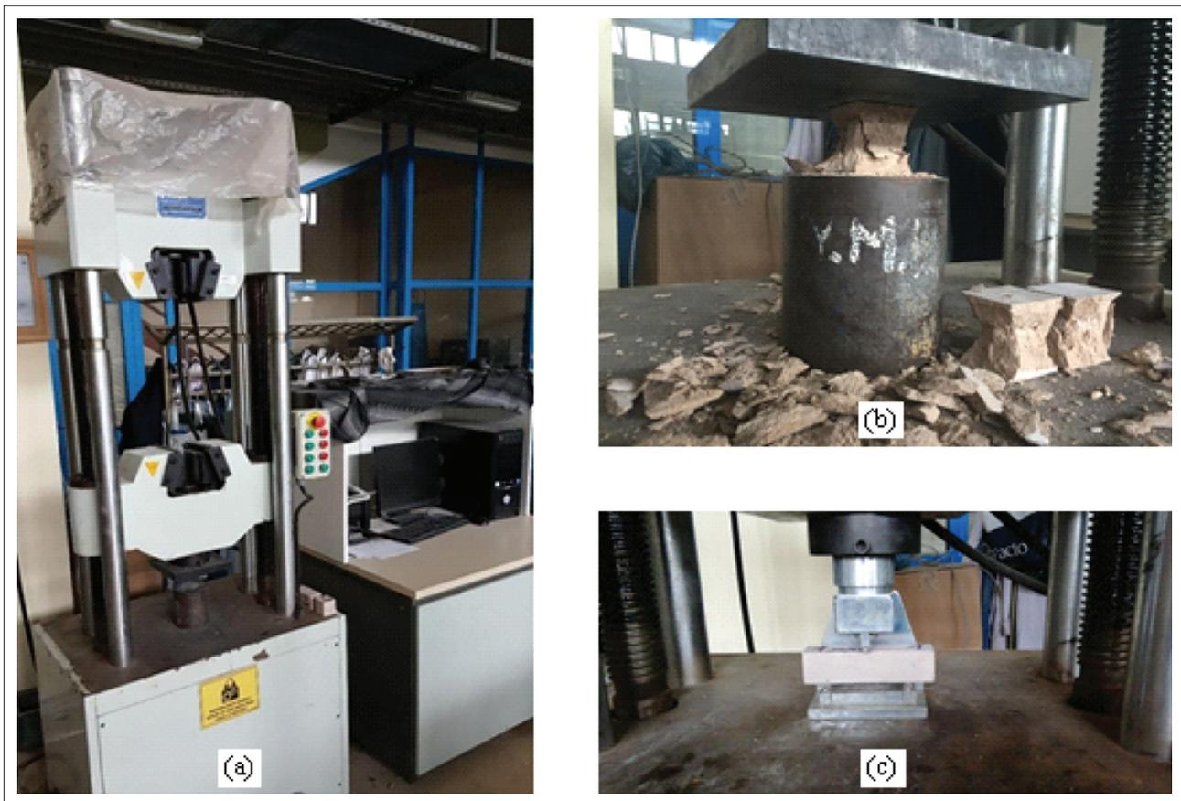
**Figure 3.** (a) Universal press, some views from (b) compression tests and (c) three-point flexural tests.
