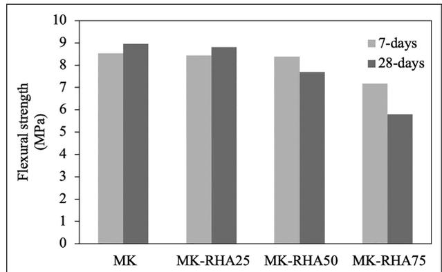
Figure 8. Flexural strength of geopolymer mortars at 7 and 28 days of ageing.
