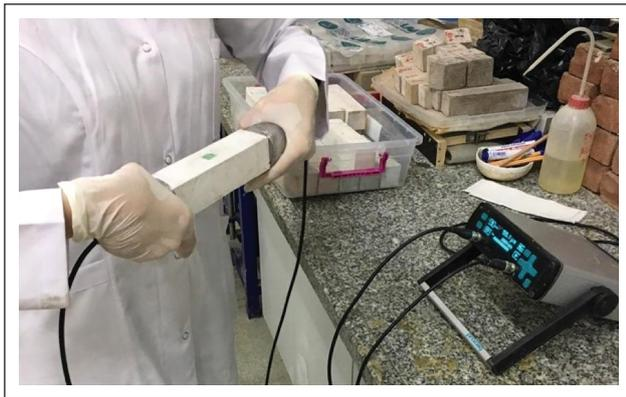
Figure 4. A view from ultrasonic pulse velocity tests.
