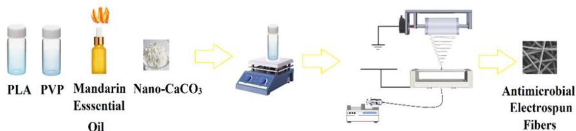
**Figure 1.** Schematic representation of the fabrication of bioactive composite electrospun webs
