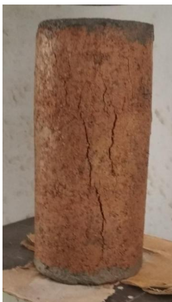
Figure 6. Typical failure pattern of rammed earth compression specimen
