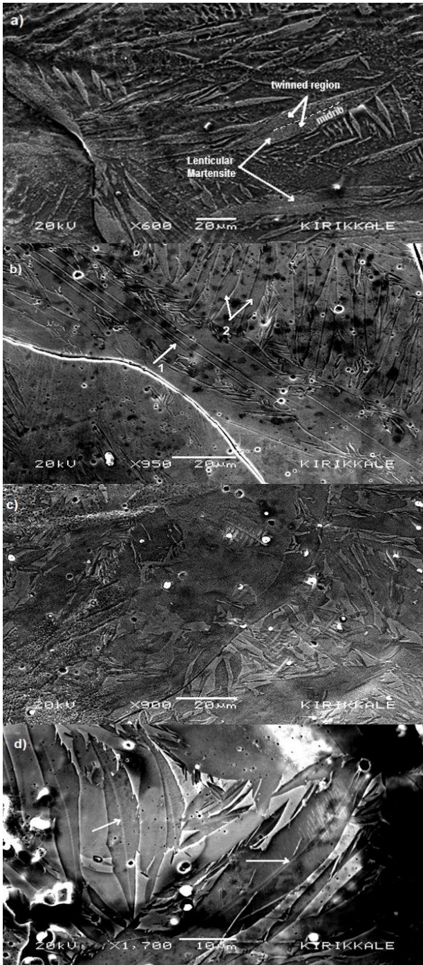
Figure 2. Thermally induced b.c.c. ( \alpha' ) martensite structures; (a-b) lath and lenticular martensite in Fe-30wt.%Ni-2.6wt.%Mo-0.8wt.%Co, (c-d) massive and lenticular martensite in Fe-30wt.%Ni-2.6wt.%Mo-1.8wt.%Co.
