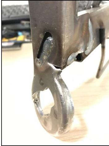
Figure 10. Rupture in the bracket that occurred during physical testing.
