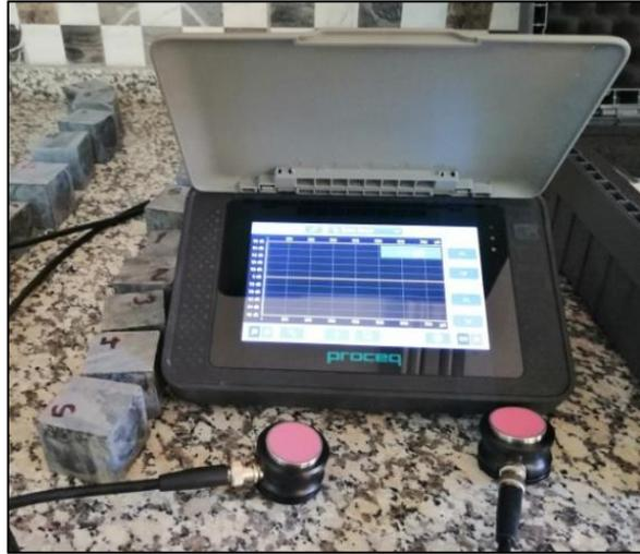
Figure 2. Ultrasonic waves tester
