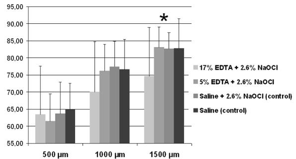
**Figure 3.** Bar graph (means and standard deviations) showing the microhardness values for experimental groups and controls at each distance ( $n = 20$ ). Asterisk (\*) indicates the distance where a statistical significance was found among groups ( $p<0.05$ ).
