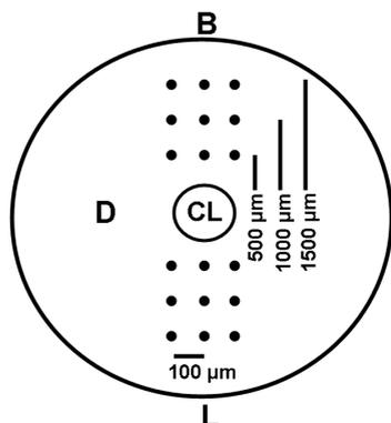
**Figure 2.** Schematic illustration of the root section, as well as the indentation points and locations in the microhardness test (B: buccal, CL: canal lumen, D: dentin, L: lingual).
