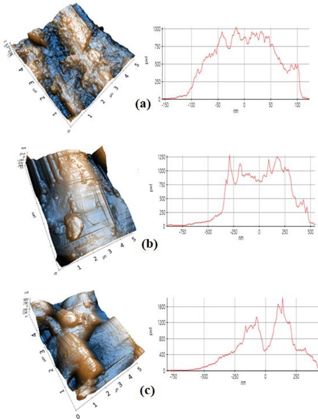
**Figure 3.** AFM Images and region histogram of Eggshell Sample (a) outer (b) inner (c) membrane
