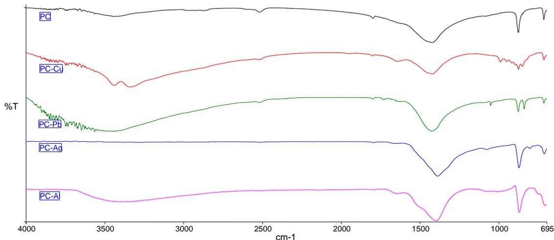
**Figure 4.** FTIR spectra of PC, PC-Pb, PC-Cu, PC-Ag and PC-Al
