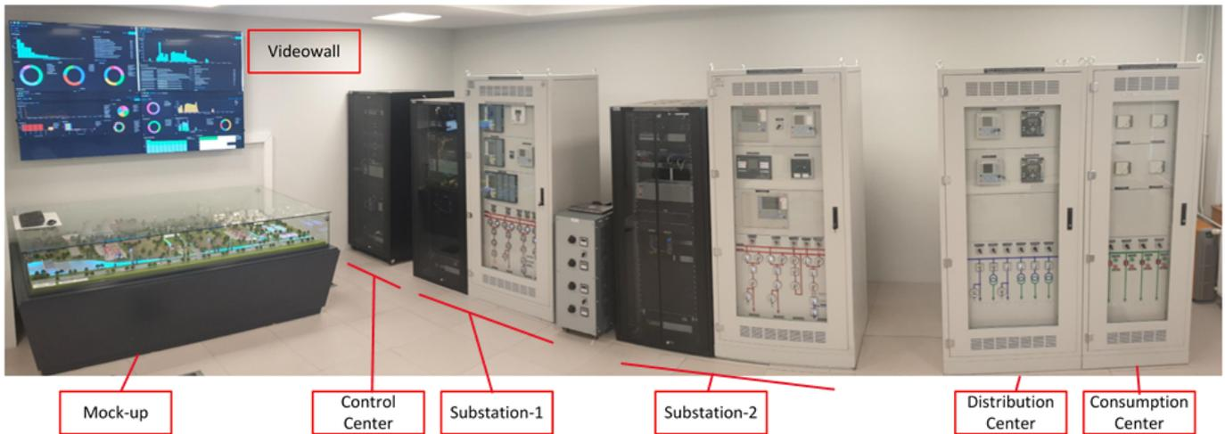
Figure 1. Physical Representation of The Energy Management Testbed Center.
