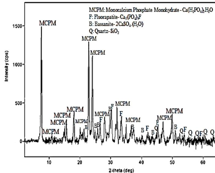
Figure 6. XRD pattern of MCPM as received
