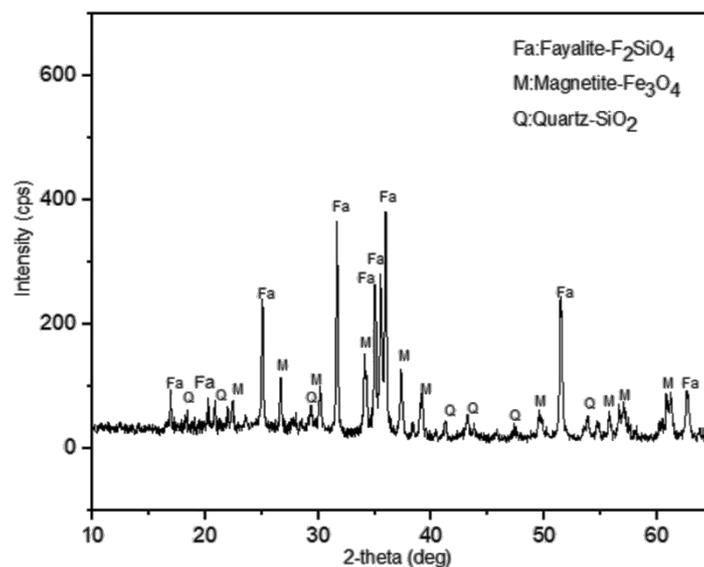
Figure 2. XRD pattern of copper smelting slag sample
