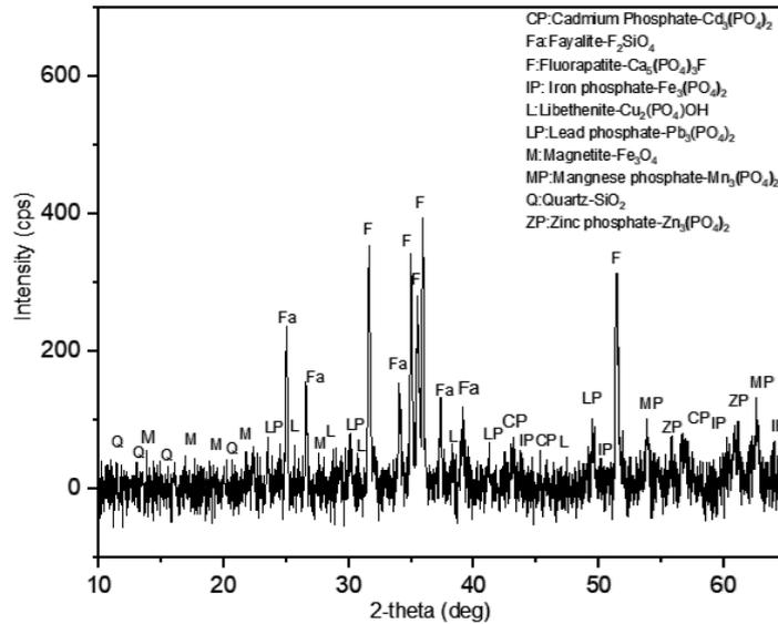
Figure 5. XRD pattern of copper smelting slag residue (Copper smelting slag treated by MCPM)
