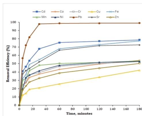
Figure 3. Effect of reaction times on immobilization of heavy metals from 25g copper smelting slag by 0.1M of MCPM.
