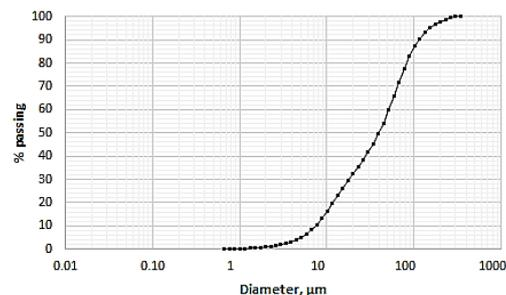
**Figure 1.** Particle size distribution of copper smelting sample.
