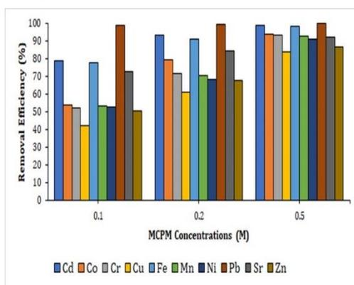
**Figure 4.** Effect of MCPM concentrations (0.1, 0.2 and 0.5 M MCPM) on immobilization of heavy metals from 25g of copper smelting slag at 180 minutes of precipitation process.
