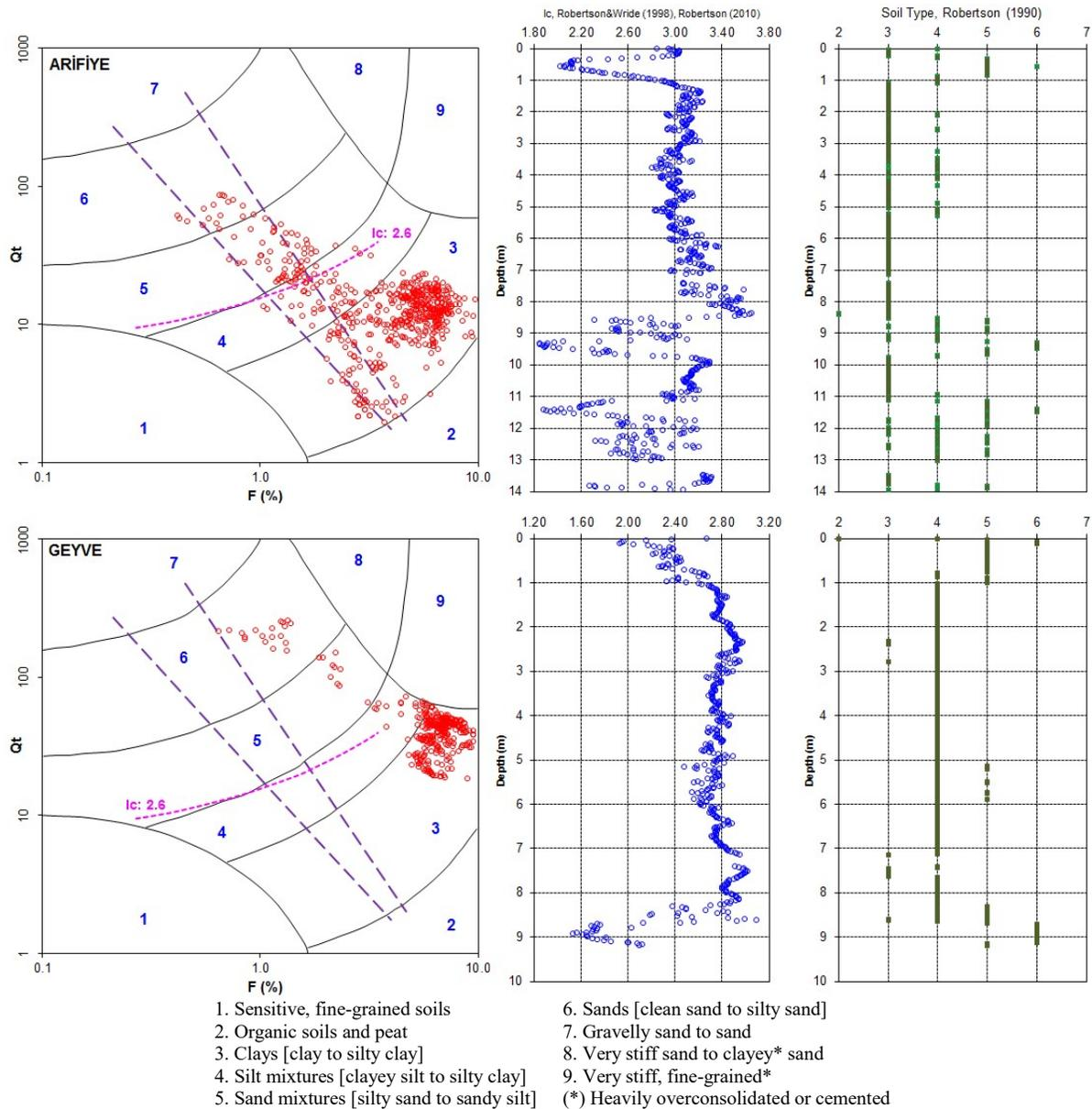
Figure 5. SPCPT sample profiles for different soil classes [23] and depth - soil type behaviour index  $I_c$  relationship [24]
