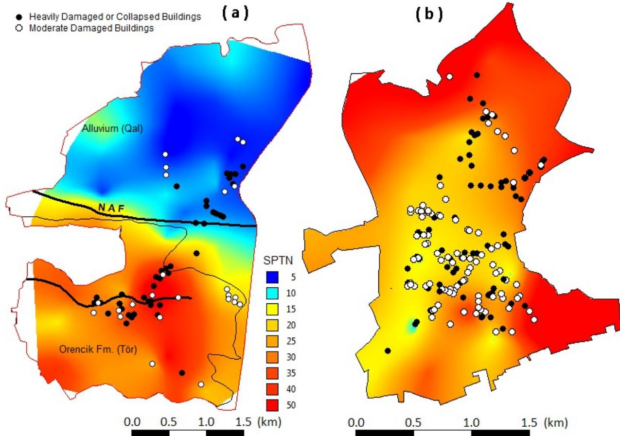
Figure 6. Standard penetration resistance maps and damage distribution (a) Arifiye (b) Geyve
