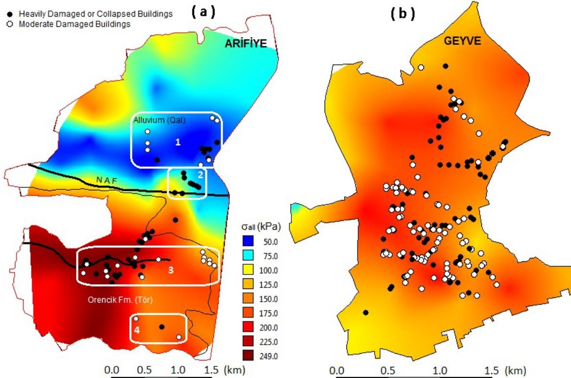
Figure 8. Allowable bearing capacity maps and damage distribution (a) Arifiye (b) Geyve
