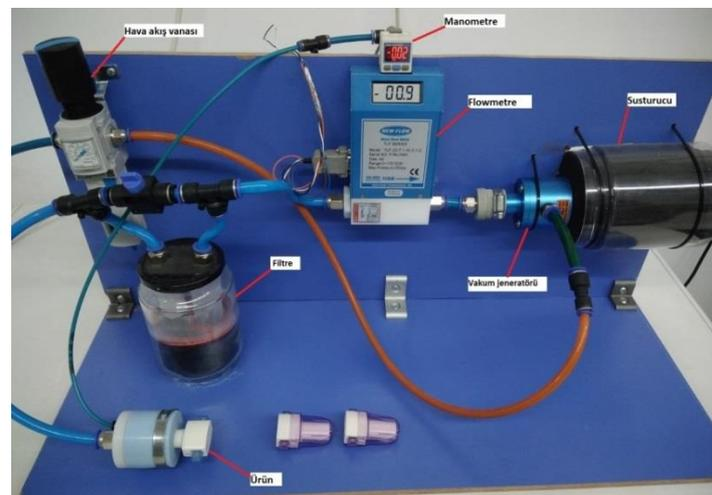
**Figure 5.** Air flow tester developed by Bimed
