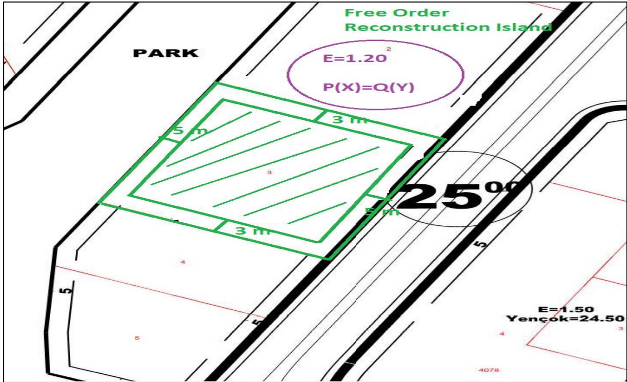
Fig. 4. Representation of the free building zoning island with a total construction area of 1.20
