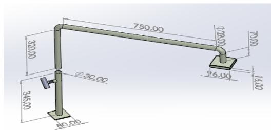
**Figure 3. Buttress of ultrasonic sensor**
