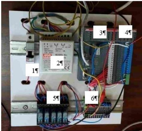
Figure 4. Control unit measuring water depth in Class A pan (1-circuit breaker 2-power supply, 3-PLC (CPU), 4-analog module, 5-relays and 6-clemens)
