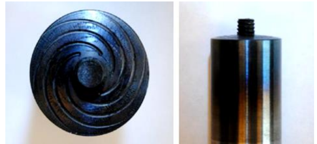
Figure 7. Tool with hollow spherical shoulder and cylindrical threaded pin [23]
