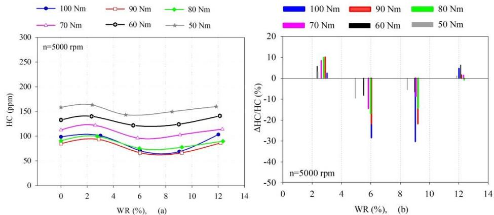
**Figure 17 (a-b).** Variations and VRs of HC emissions versus different WRs under five different loads at 5000 rpm, respectively.
