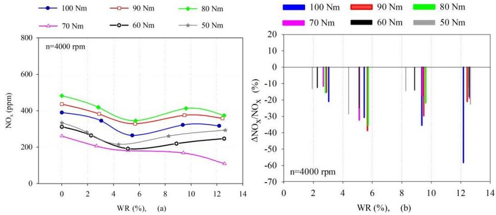
**Figure 12(a-b).** Variations and VRs of NO<sub>x</sub> emissions versus different WRs under five different loads at 4000 rpm, respectively.
