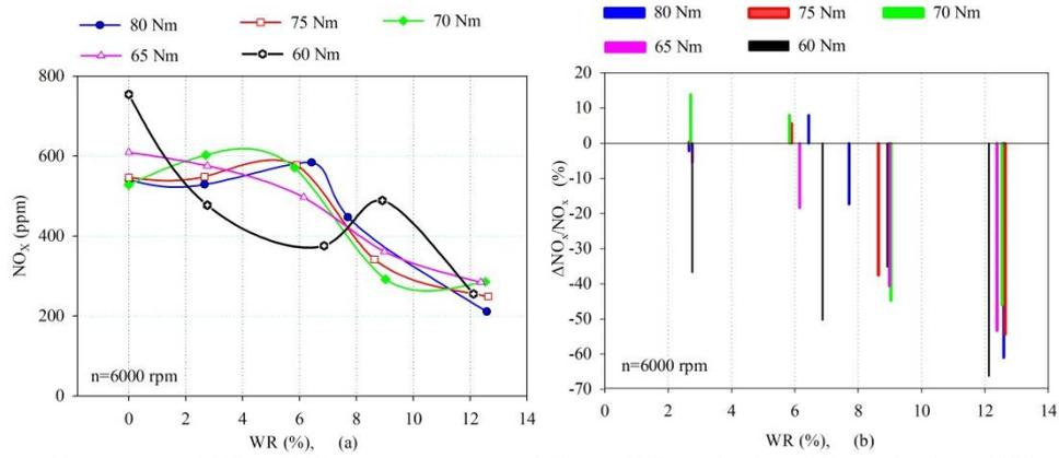
**Figure 14 (a-b).** Variations and VRs of NO<sub>x</sub> emissions versus different WRs under five different loads at 6000 rpm, respectively.
