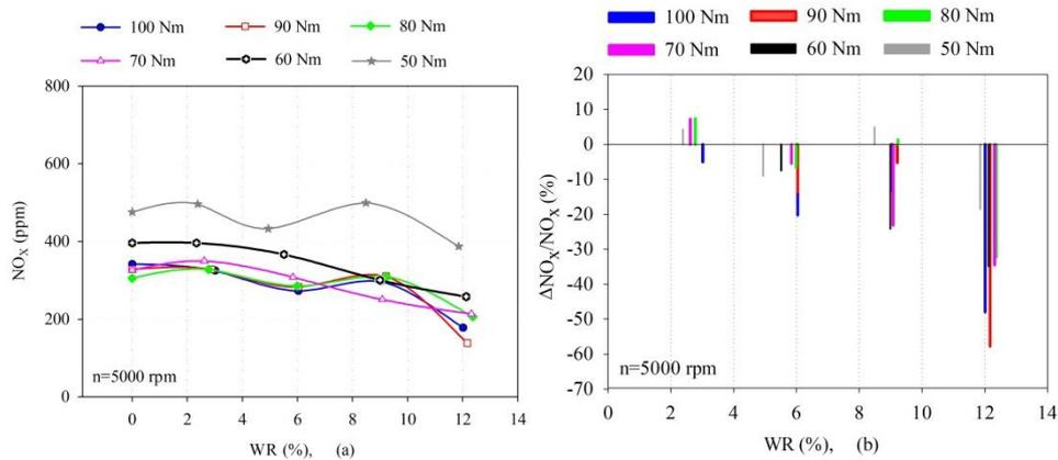
**Figure 13 (a-b).** Variations and VRs of NO<sub>x</sub> emissions versus different WRs under five different loads at 5000 rpm, respectively.
