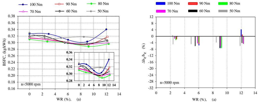
Figure 5 (a-b). Variations and VRs of BSFC versus different WRs under five different loads at 5000 rpm, respectively
