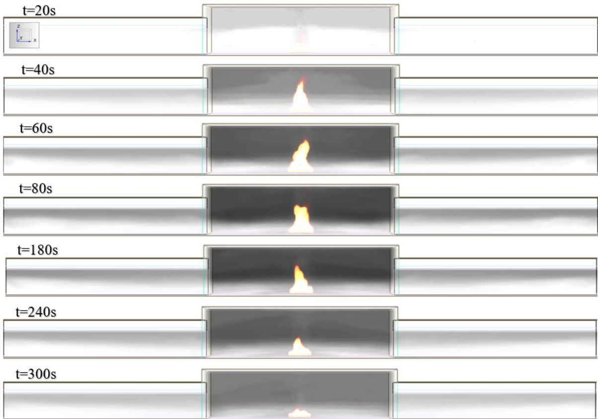
Figure 12. The soot distribution along the station during fire
