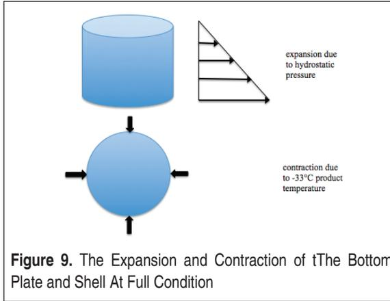
stress. The stress also causes the change in diameter. According to API Standard 653, the pressure applied to the shell near the bottom plate is calculated as 126 MPa using Eq. 4. Here,  $D$  is the diameter of the tank in feet,  $H$  is the height of the product in feet,  $G$  is the specific gravity of the product (0.68), and  $t$  is the wall thickness of the first shell in inches.
