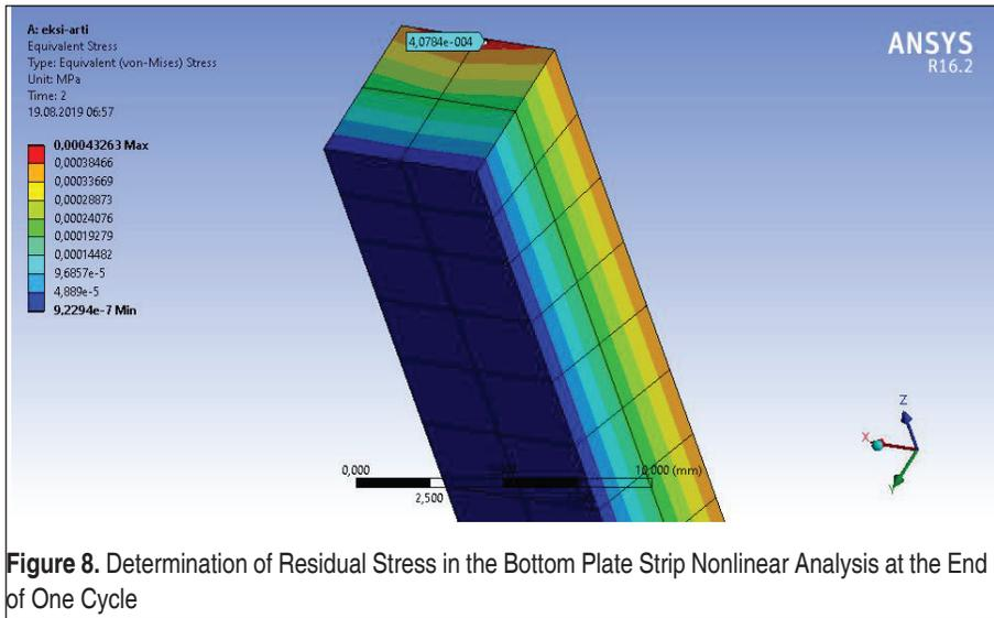
much at the wall (shell) level. The 157 MPa principal stress encountered in the 6 mm thick bottom plate or the 190 MPa obtained in terms of the von Mises stress is below the level that will cause plastic deformation, considering that the yield strength is 220 MPa.
