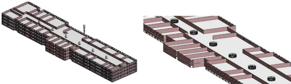
Figure 34. The increase in the cross-section of the dirty air outlet chimneys on the floors and the settlement points inside the building were drawn in Revit 2016 software (Tohidi, 2022).
