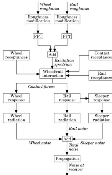
**Figure 1.** Schematical diagram of TWINS model [32]
