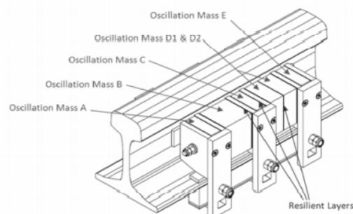
**Figure 2.** Isometric view of tuned rail damper [58]
