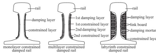
**Figure 3.** Monolayer, multilayer, and labyrinth constrained rail dampers [59]
