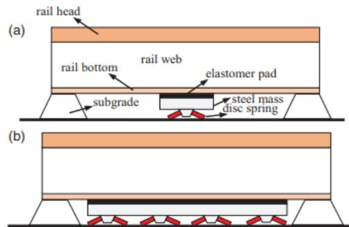
**Figure 6.** DVA structure along the track a) discrete arrangement and b) continuous arrangement [83]
