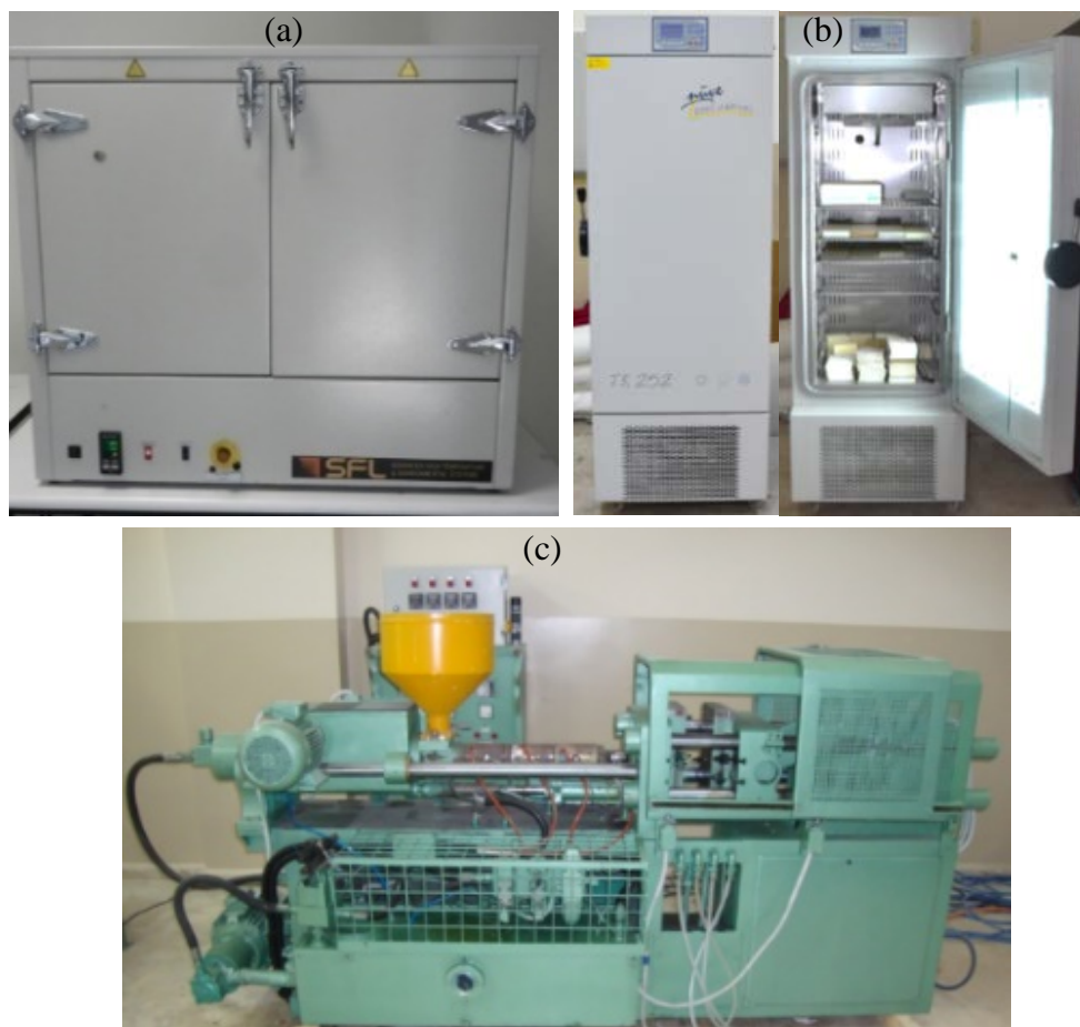
Figure 2. Devices used in production a) oven, b) conditioning unit and (c) plastic injection machine
