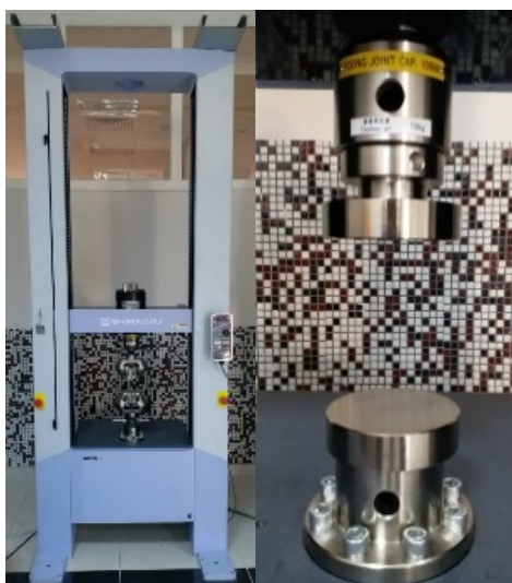
Figure 3. Shimadzu AGS-X 100 kN universal tensile-compression tester and compression plates
