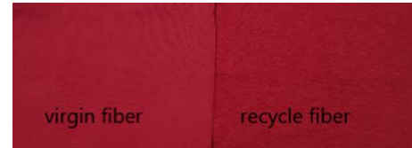
Figure 1. Photos of fabric sample produced by using virgin and recycled fiber
