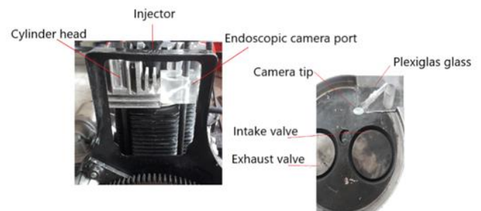
Fig.1. Modified cylinder head for cold flow testing
