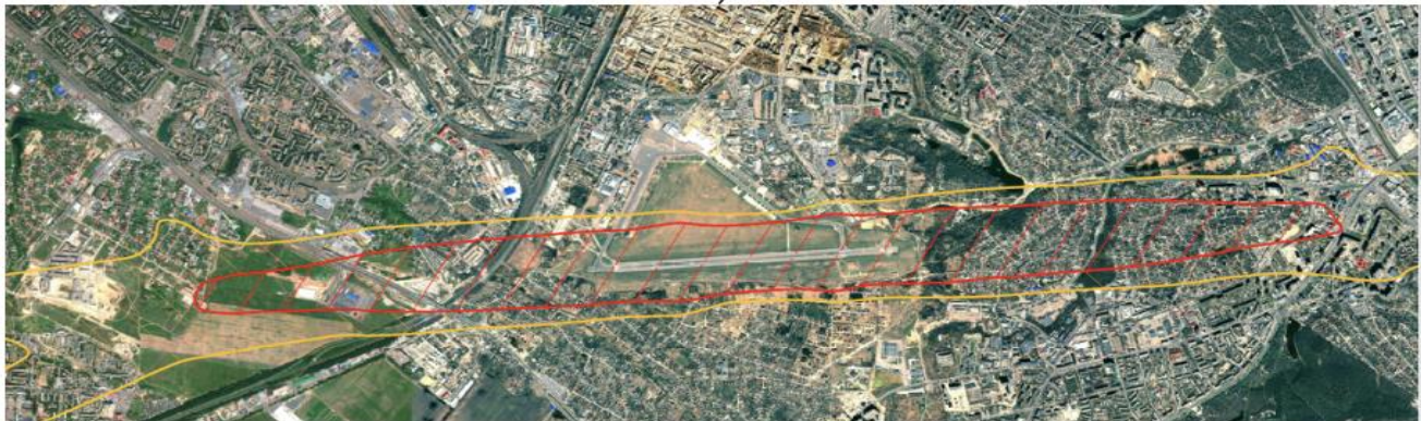
Fig. 3: Airport Kyiv/Zhulyany: a) the apron with aircraft stands near the terminal is located at a distance of more than 1 km from the runway axis; b) noise zones for 2010–2020 air traffic scenario – red contour is for L_{eq\ day}=65\ dBA
