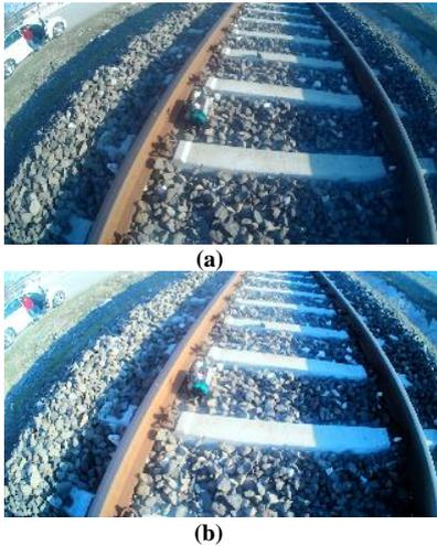
**Figure 3.** Histogram Equalization (a) Original Image b) Histogram Equalized Image
