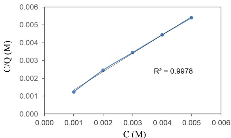
**Figure 6.** Langmuir adsorption plot of MS electrode obtained in 0.5 M HCl containing various concentration of 2I4MTA5C
