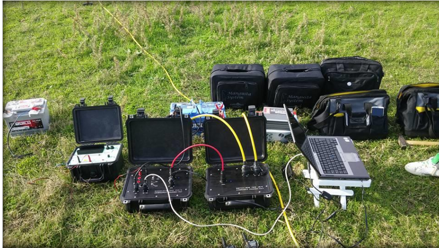
Figure 4. Ambergeer brand, Mangusta TMG 255 E model multi-electrode (48 electrode capacity) resistivity tomography device
