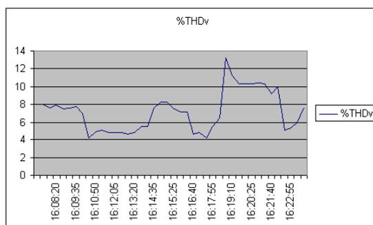
**Figure 6.** Real time harmonic measurement values.
