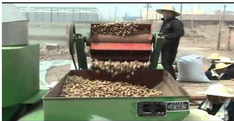
Figure 2. Mechanized shelling ( Walke et al., 2017 ).
