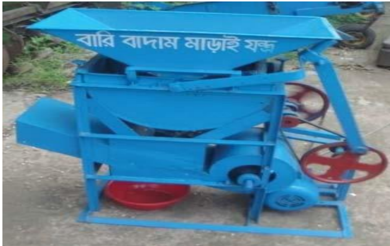
Figure 6. Groundnut sheller by Hoque and Hossain (2018) .
