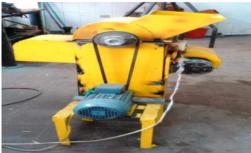
Figure 5. Prototype Groundnut sheller by Madi (2017).
